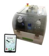
Our latest Acid decapsulation system, the **iSA700DCTM**, is the first negative pressure decapsulation system available in the market. No more acid projection, possibility to decapsulate device on PCB, easy control with our iPanel<sup>TM</sup> interface, and many more advantages ...
